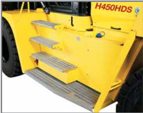
Broad running boards
