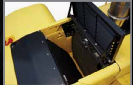
Hinged cover enables easy serviceability access to radiator cooler
