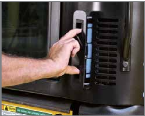
Easily accessible interior cabin filter
